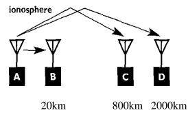
A to B = Recommended working frequency is 3 MHz
