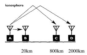
A to B = Recommended working frequency is 3 MHz
